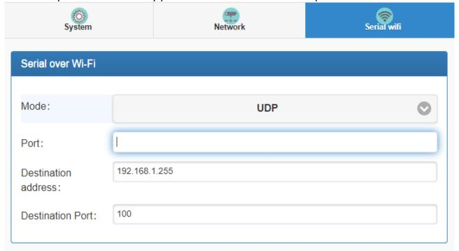
Clients like Link2AIS then will receive the serial data stream on port 100.
