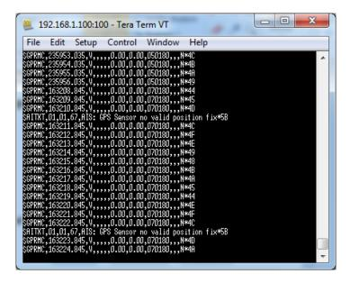
If the sentences are incomplete or do not show as expected, please first make sure the entered Baud rate is correct for both the Nauticast W1 and the serial device..
